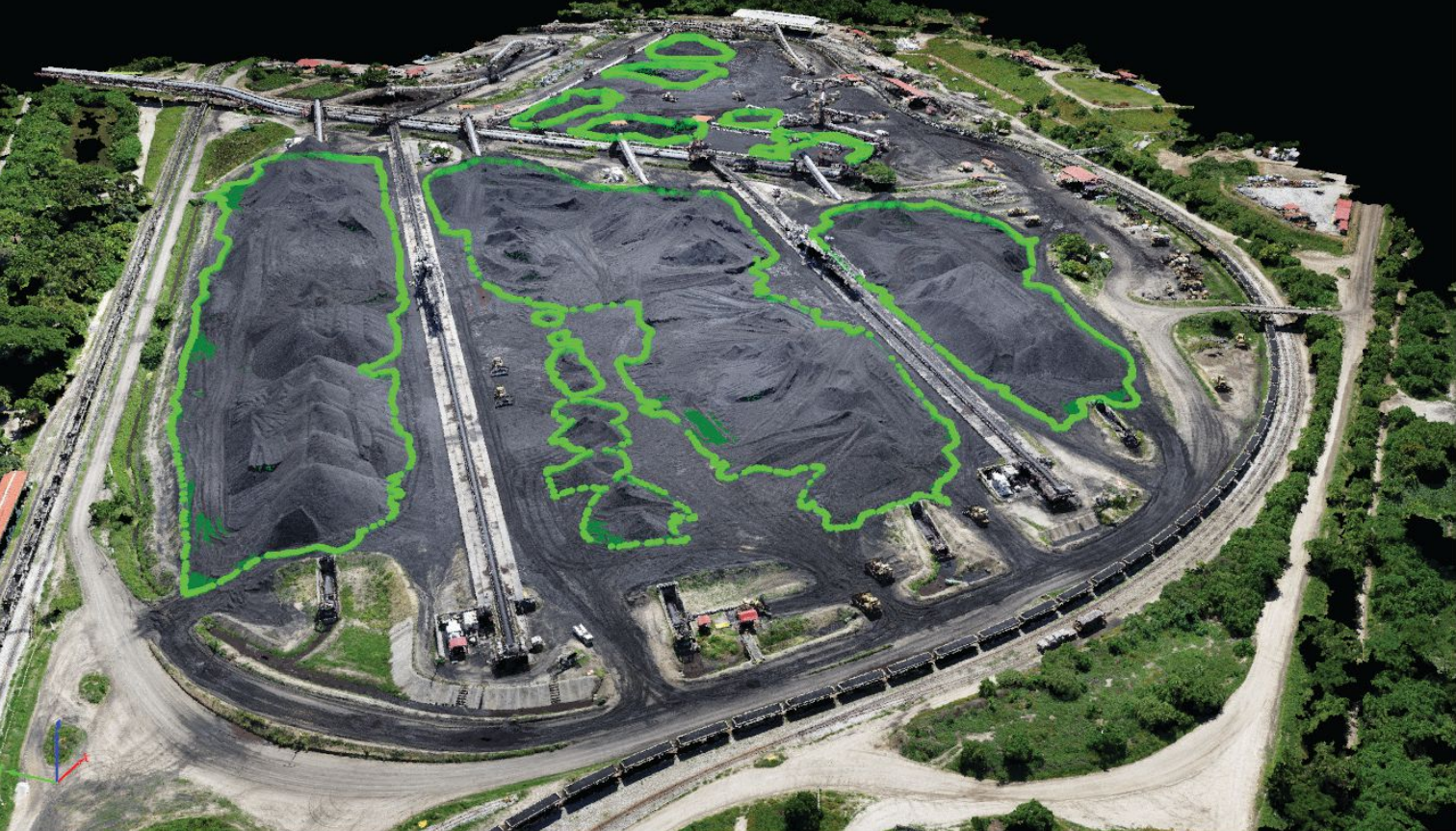
Drones can be used for a range of applications at the mine, including surveying, mapping, exploration, stockpile management, reaching inaccessible areas, waste and water management, and mining environmental protection. Pictured: an eBee X mapping dataset from a Colombian mine. Photo: AgEagle
