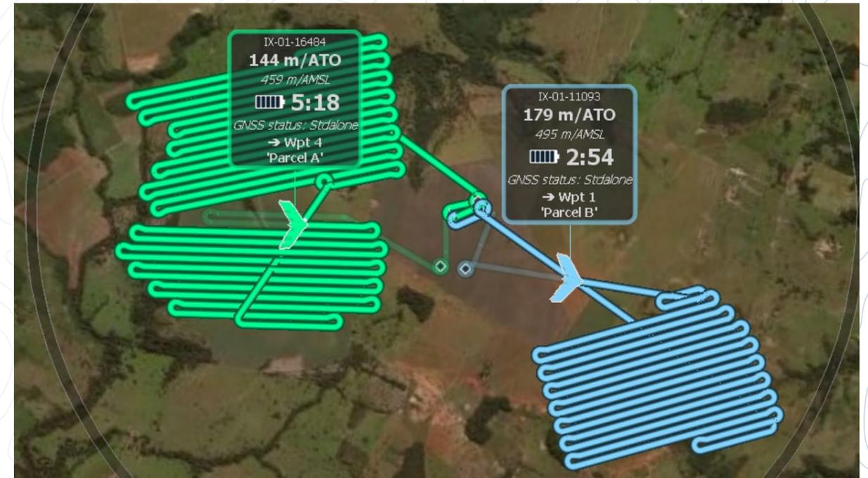
With eMotion, flights are built using mission blocks. Just choose your block, highlight the region you want to map, define key settings, and eMotion auto-generates your drone's flight plan. Multi-flight missions are supported and you can activate/import elevation data for even safer, terrain-accurate flights.
